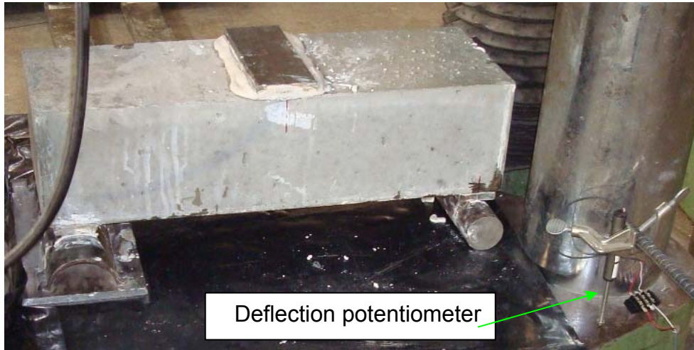
Figure 3.24 Test setup and deflection transducer
