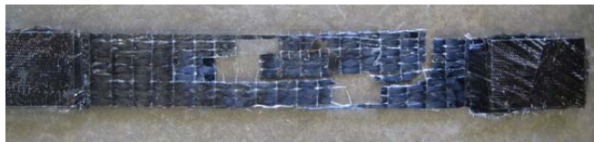
Figure A.3 Failure of coupon C-3
