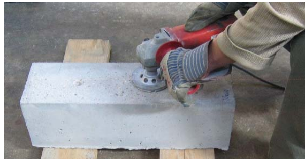
Figure 2.18 Preparing the concrete surface [Courtesy of Insung Kim]
