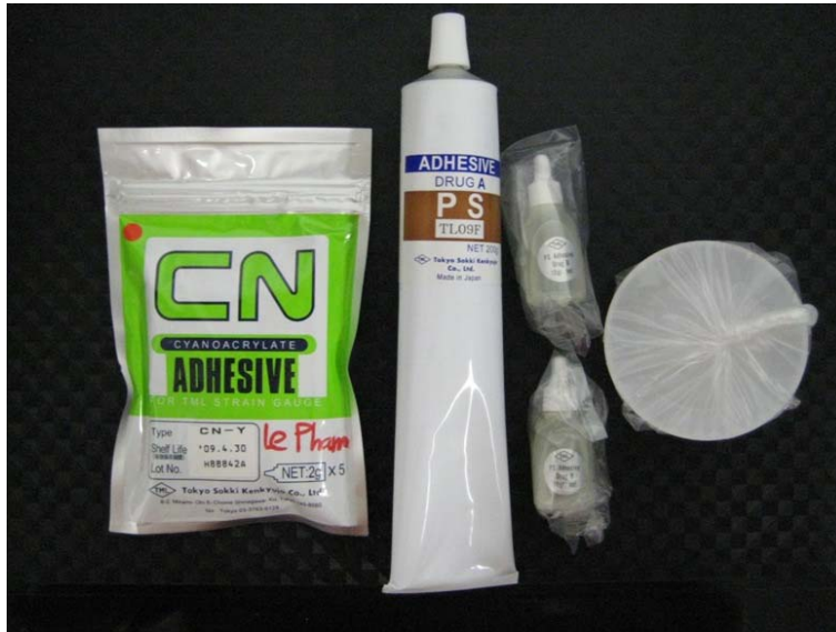
Figure B.1 Adhesives for installation of strain gages to CFRP
