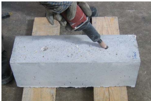
Figure 2.20 Rounding off the edge of the holes and checking with a radius gage
