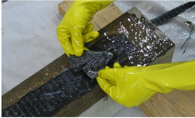
Figure 2.28 Fanning the end of CFRP anchor
