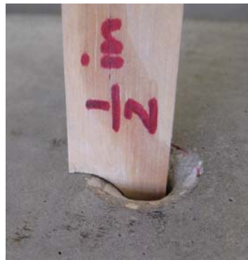
Figure 2.20 Rounding off the edge of the holes and checking with a radius gage
