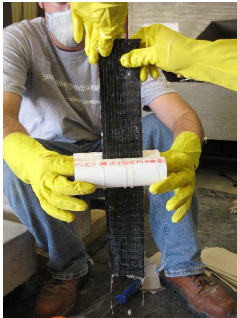
Figure 2.25 Rolling CFRP sheet through PVC pipes
