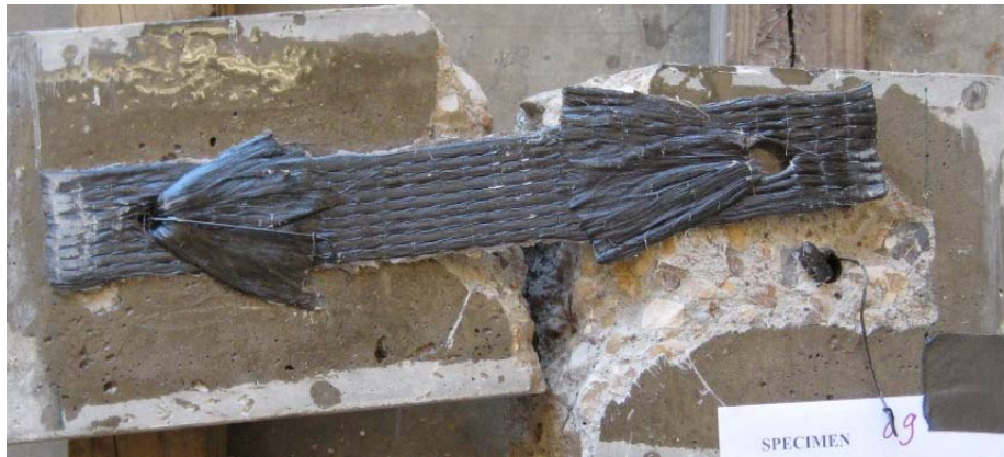
Figure 3.11 Detail of fractured CFRP anchor
