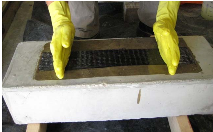
Figure 2.26 Applying and aligning CFRP sheet
