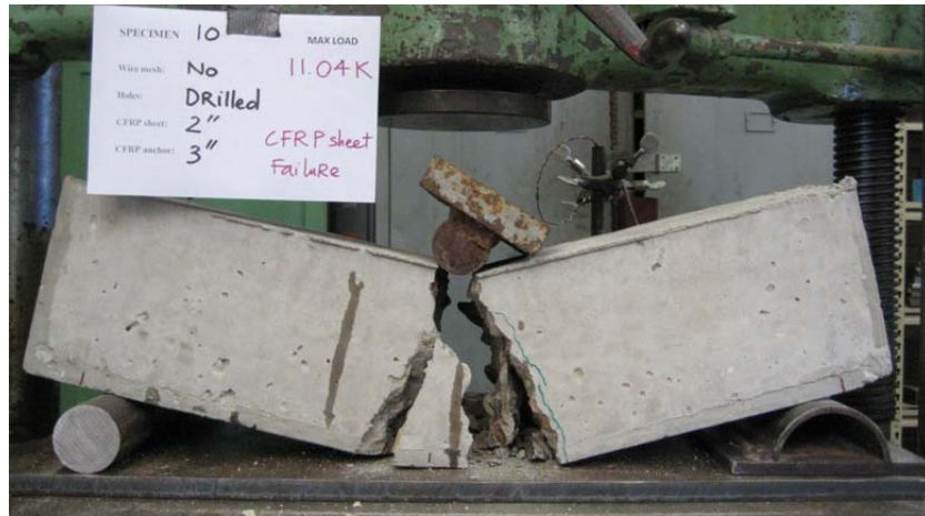
Figure 3.8 Fracture of CFRP sheet
