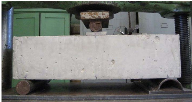
Figure 3.7 Testing beam specimens
