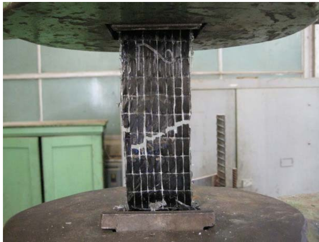
Figure A.2 Failure of coupon C-2
