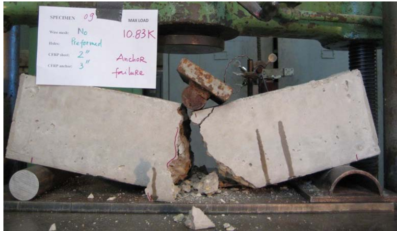
Figure 3.10 Fracture of CFRP anchor
