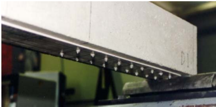
Figure 2.3 Mechanically fastened prepreg CFRP plate [Lamanna, 2002]
