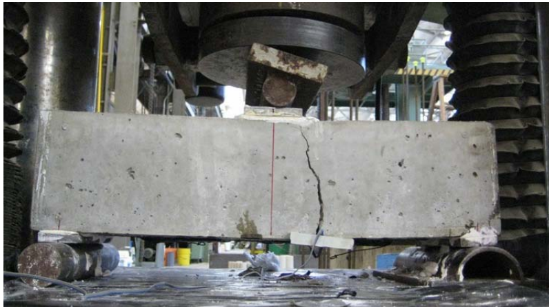
Figure 3.28 Failure caused by anchor debonding
