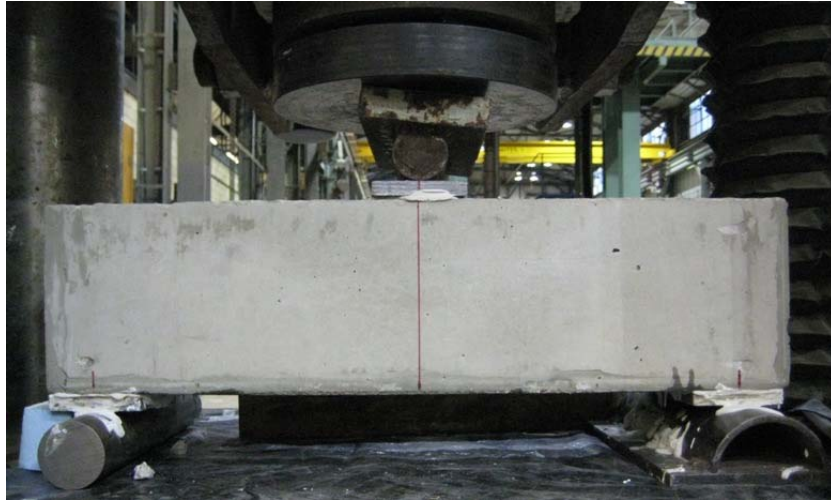
Figure 3.18 Test setup with bearing plates
