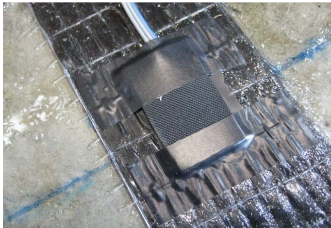
Figure B.12 Cover the gage for protection
