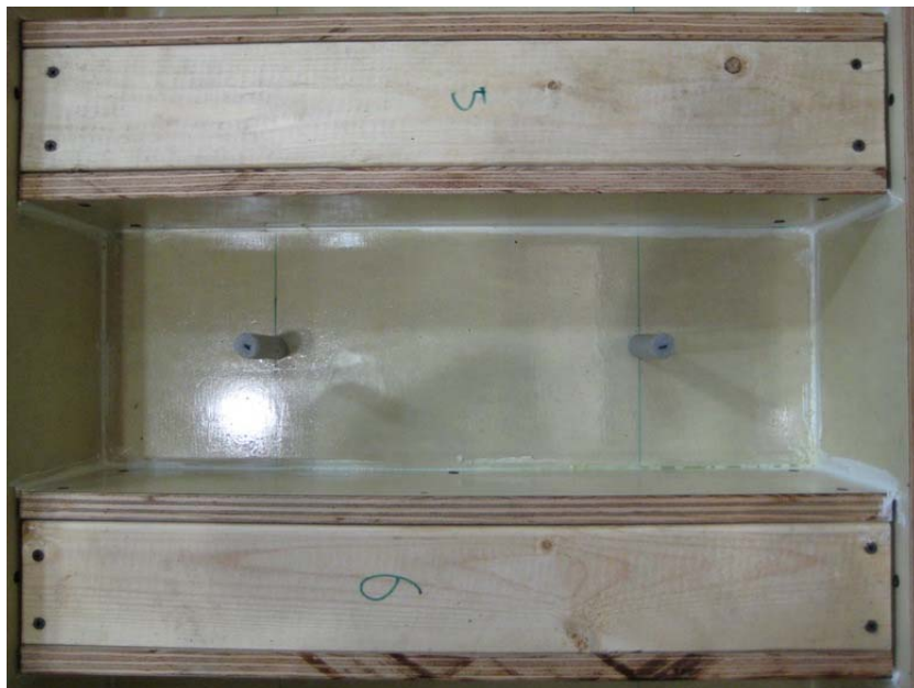
Figure D.3 Pre-formed holes using backer rods
