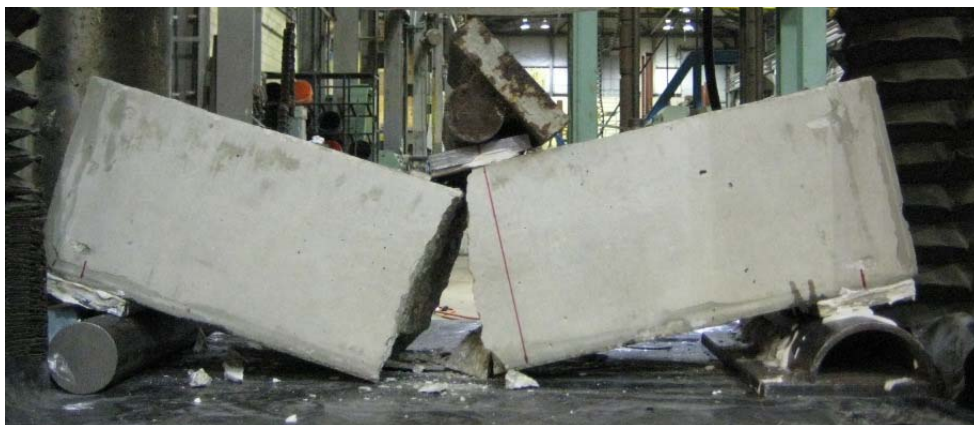
Figure 3.19 Failure caused by anchor fracture
