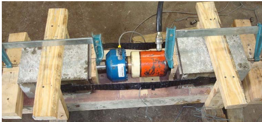
Figure 3.42 Blocks held down by wood frames
